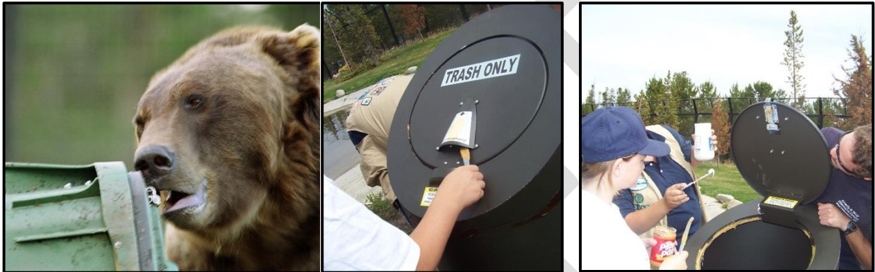
Figure 4. Small amount of bait applied to latches and inside rim of products.
