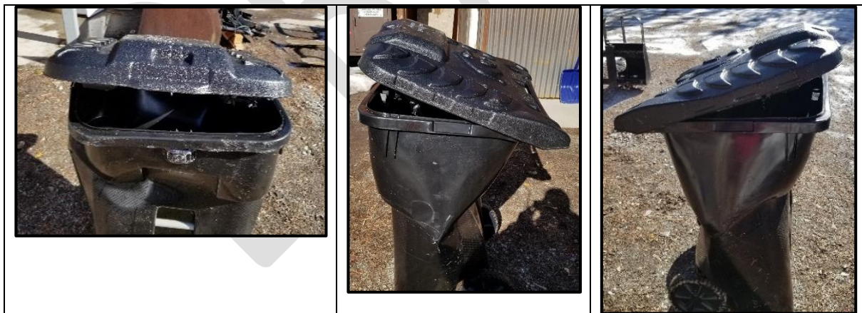
Figure 5. Photos illustrating damage to products that render them non-functional.
