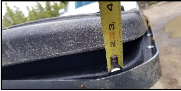
Figure 6. Measuring the gap between the lid and cart body that was created by the bears.
