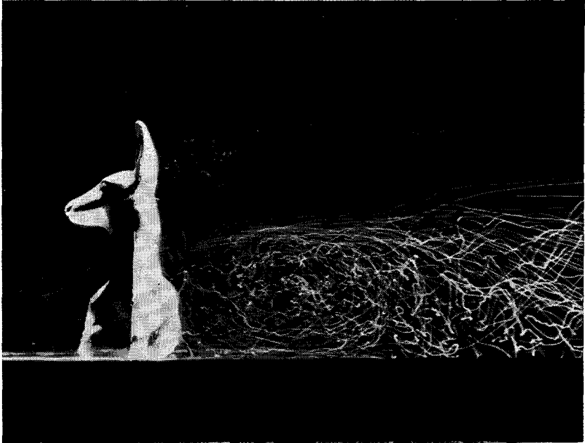
Figure 2.—Patterns of air flow about a model of a deer in a bedded posture in the Thermal Environment Simulation Tunnel. Note the turbulent area that develops on the leeward side of the animal.
