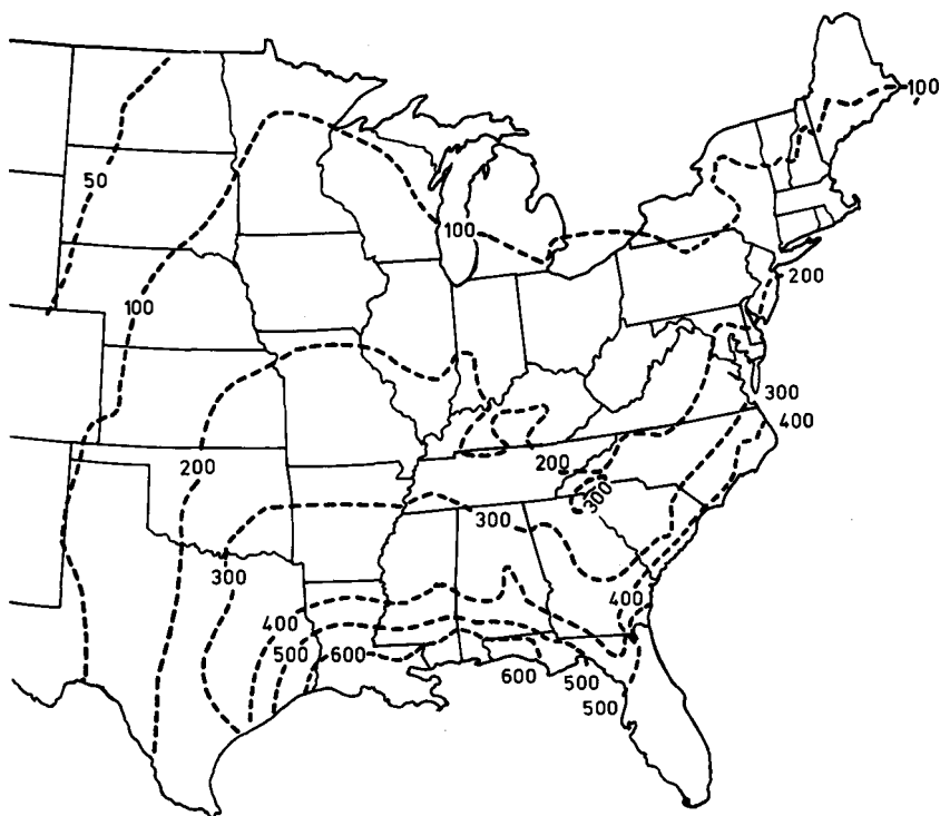
Figure 5. Average annual values of the rainfall factor, R , for areas of the United States east of the Rocky Mountains (from Wischmeier and Smith 1965). See text for explanation.
