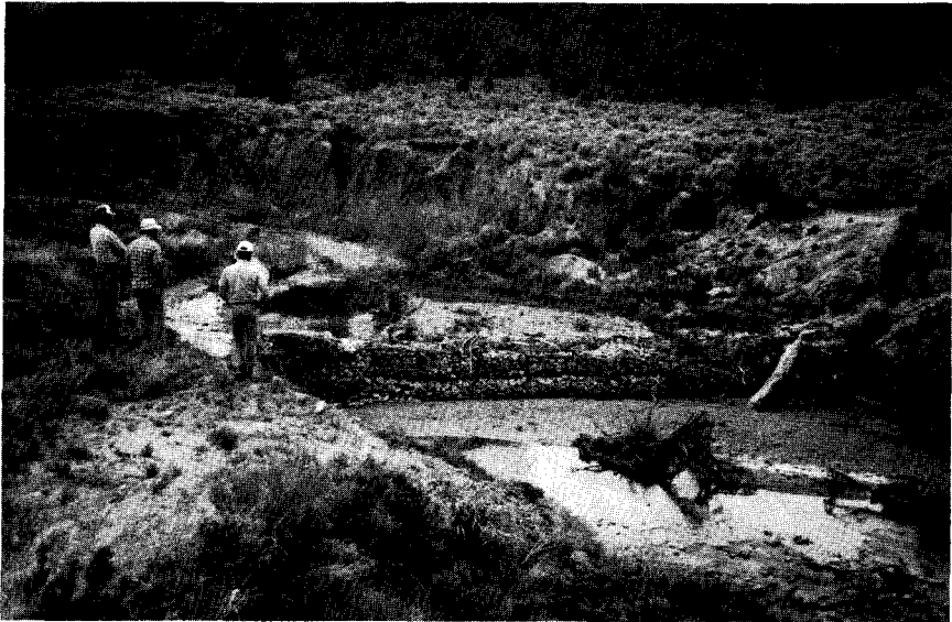
Figure 2. Inappropriate design and placement of a low check dam in a Condition C channel.
