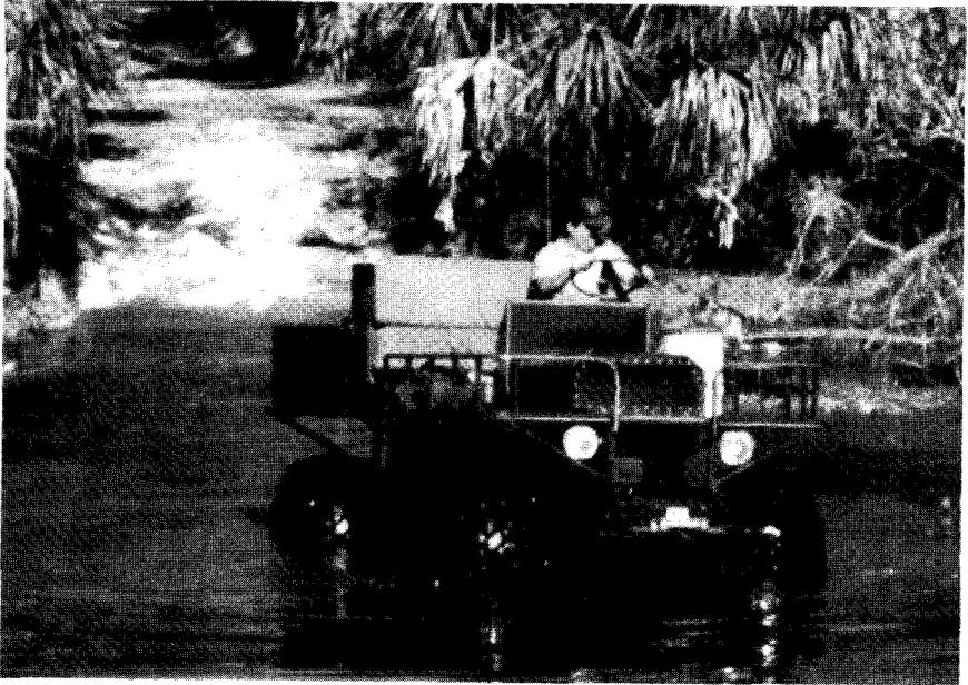
Figure 2. Homemade swamp buggy designed for off-road travel through a wide variety of hydrological, soil and vegetation conditions encountered in the Big Cypress region.
